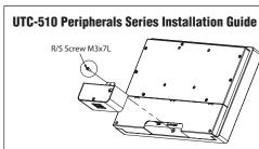
Customer can easily attach the peripheral by re-using the screw that was taken out from Frame.
