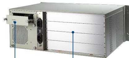
Built-in alarm board (MIC-3924L-AE)
